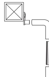
**STEP 1** - Handrail component designed for use where a gate has been installed on a post and secondary handrail needs to be installed on the same side of the post. See illustration above.
