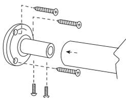
**STEP 1** - Slide Level Wall Bracket onto straight handrail.
