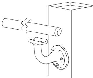
**STEP 1** - Determine proper bracket height and orientation for angle of rail.
