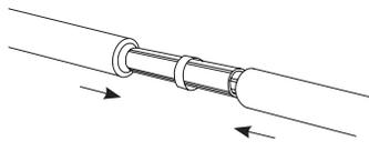
**STEP 1** - Beauty rings can be used to conceal cut rails at each straight joint of handrail.
