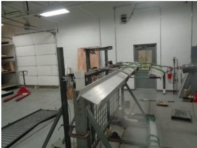
Photo No. 6 Horizontal Uniform Load on Top Rail
