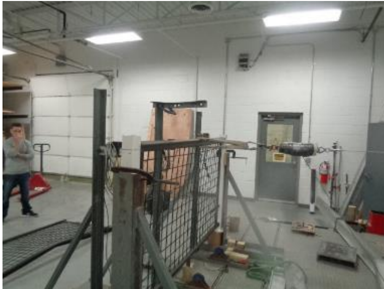
Photo No. 4 Horizontal Concentrated Load Test at Midspan of Top Rail
