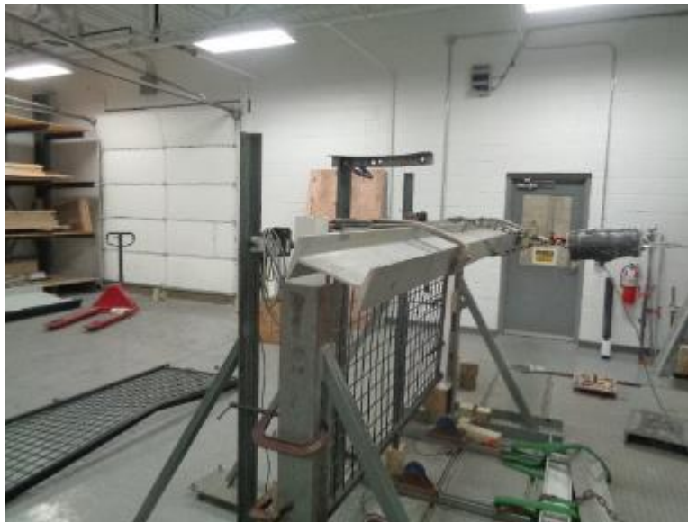
Photo No. 5 Concentrated Load at Ends of Top Rail (Brackets)
