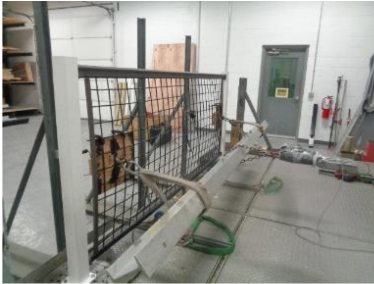
Photo No. 3 Infill Load Test at Edges of Infill
